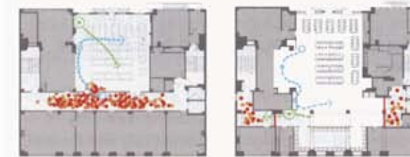
To open the congested floor, the food pick-up line was reversed, relocating the forming line away from central corridor traffic.
